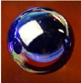
Fusion fuel is encased in a sphere of high density carbon (synthetic diamond) the size of a pepper corn
