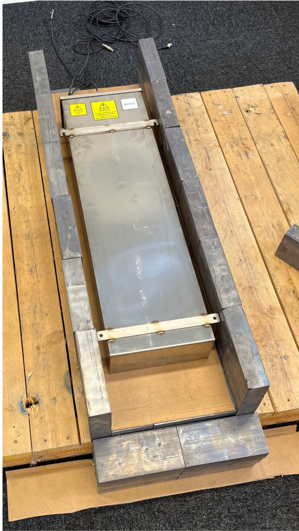
Above: Photograph of the partial construction of the lead producer layer. The lead was assembled on all six sides of the N50L module.
