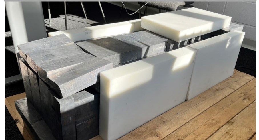
Above: Photograph of the lead sarcophagus with partial construction of an outer reflector layer constructed of 50 mm thick high-density polyethylene.
