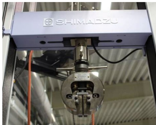
10kN static load frame
